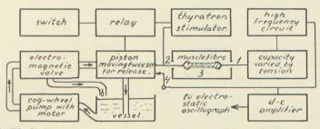
Fig. 8. Block diagram of the arrangement for recording work diagrams during release contraction. (1) and (2) pairs of micro-tweezers to hold tendon ends of fibre. (3) muscle fibre. (4) contact recording 5 mm movement of piston and tweezer (2).
