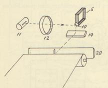
Fig. 4. Photographic recording of coil movements.
